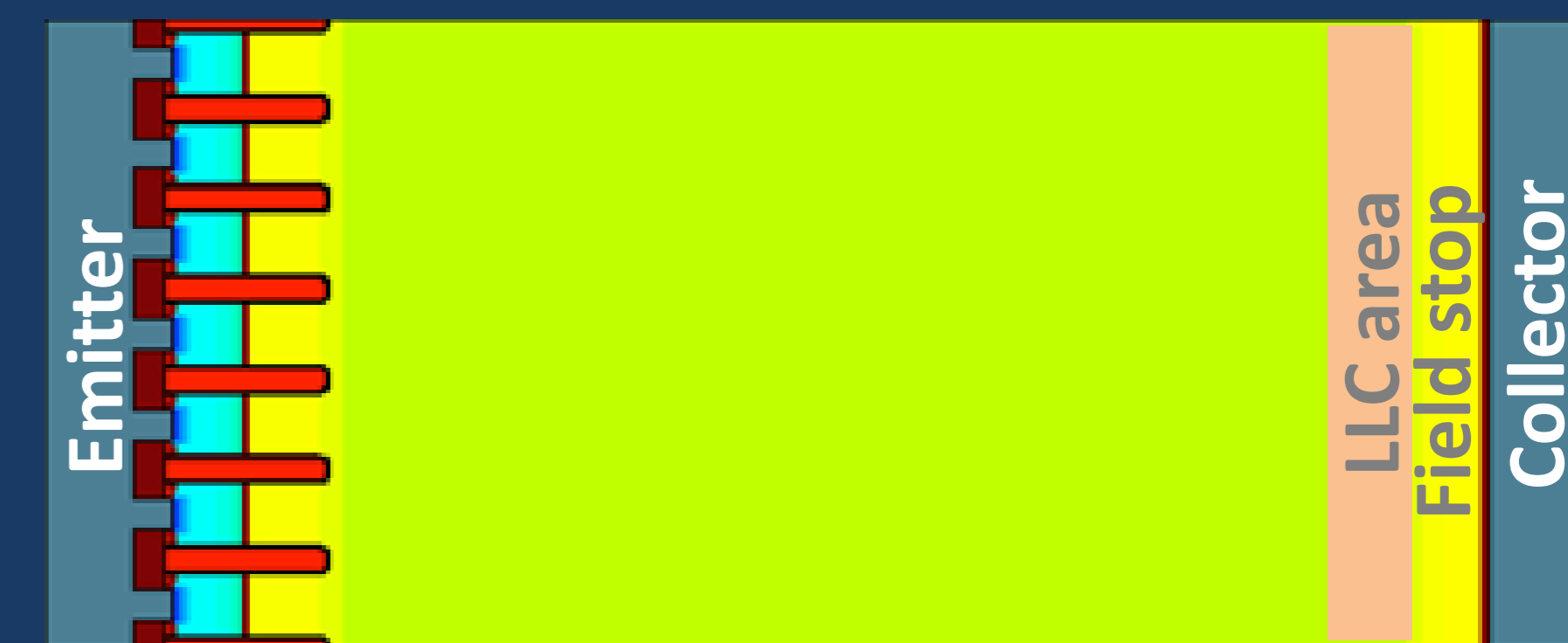
TIGBT active cell with LLC area generated by helium implantation at field stop layer
