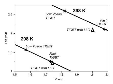
Fig. 3:  $E_{off}(V_{ceon})$  trade-off chart for Low Vceon TIGBT, Fast TIGBT and TIGBT with LLC for 298 K and for 398 K (real measurement data). All three devices were manufactured with an identical active cell and field stop. Low Vceon TIGBT and TIGBT with LLC were processed with the same collector dose. Fast TIGBT was processed with a lower collector dose.
