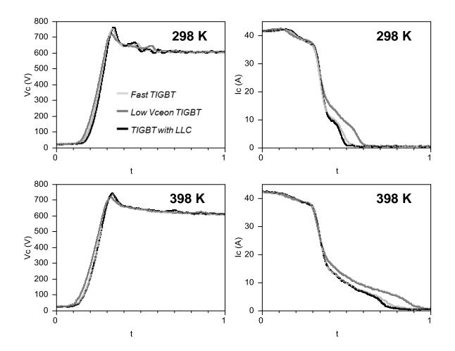
Fig. 2: Switching waveforms during turn-off for 298 K and for 398 K (real measurement data).
