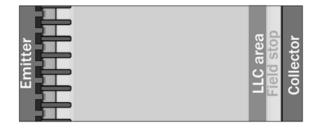
Fig. 1: TIGBT active cell with LLC area generated by helium implantation at field stop layer.
