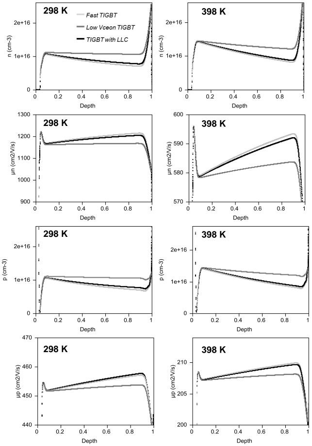
Fig. 4:  $n, p, \mu_n, \mu_p$  profiles for three types of TIGBTs (TCAD simulation).
